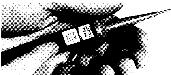
Fig. 3 — The pushbutton on the Safety Leakage Probe is depressed when the actual value of leakage current is to be read on the meter.
